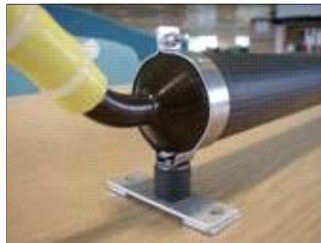
Rear exhaust mount as used on my Angels Shadow. Retaining clip made from a large Hose clip, with a cylindrical rubber mount obtained from RS components. Sandpaper is glued inside of clip to grip the carbon pipe without crushing it.
